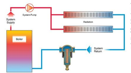
TDN models may be installed in horizontal or vertical piping. Rotate the adjustable connection such that the flow is in the direction of the arrow. "X" pipe diameters of straight run before and after the unit are not required.
