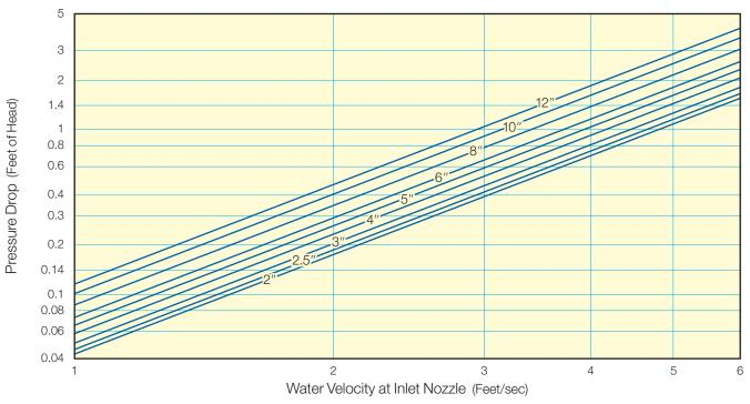
At rated flows pressure drop for 1" to 2" brass models is 0.50 feet.
