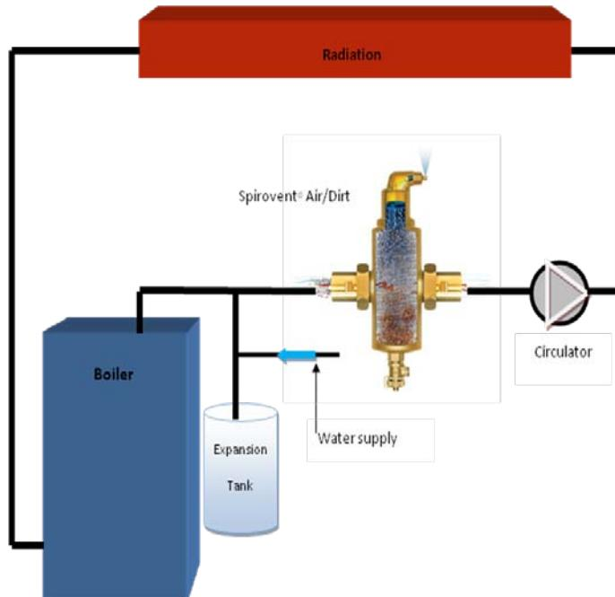
VDR models must be mounted in a straight run of horizontal piping in a perfectly upright position to allow the vent to operate freely. "X" pipe diameters of straight run before and after the unit are not required.
