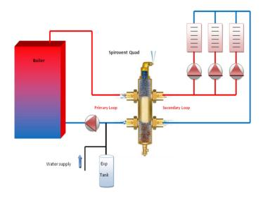
Units must be mounted in straight runs of horizontal piping in a perfectly upright position to allow the vent to operate freely. The piping normally supports the weight of the Spirovent units up to and including 12". Support legs recommended for units 14" and larger. "X" pipe diameters of straight run before and after the unit are not required.
